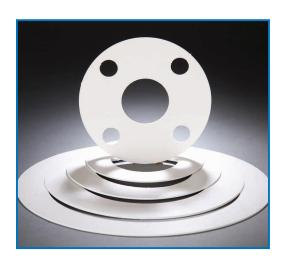
Style 5002 is 100% expanded virgin PTFE that is extremely soft and very compressible. Style 5002 has unlimited shelf life and can be removed at anytime from the flange surface since it is a non-stick product.
